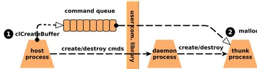
Figure 7: The interaction between host and device.
